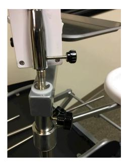
7. Align the backrest support rod with the adjustment block as shown. Compress the adjustment block to allow the support rod to travel through the block. Release the handle to lock the backrest in place. Adjustment block must remain centered to allow the support rod to travel freely.
