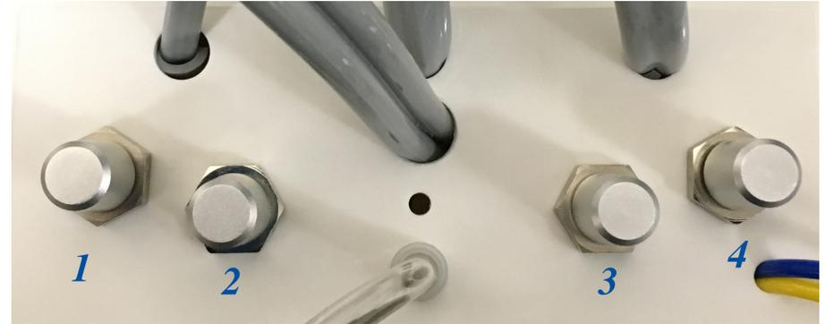
1. High speed HP air adjustment: Use this adjustment knob to adjust the amount of drive air being supplied to the selected HP.
