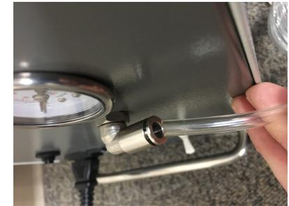
Attach the delivery unit to the compressor case as shown utilizing the included mounting tabs.
