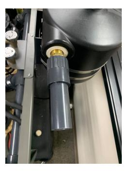
8. Install the water line to the water line port on the bottom of the separator canister. Install the drain line from the separator. Secure with the supplied hose clamp.
