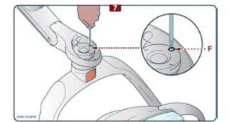
Tighten the safety screw (F) until the proper head rotation resistance is obtained.
