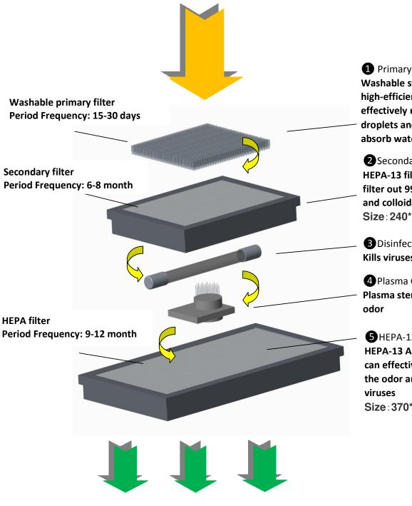
Primary Filter Washable synthetic fiber, high-efficiency filter can effectively remove the droplets and aerosol particles, absorb water vapor
