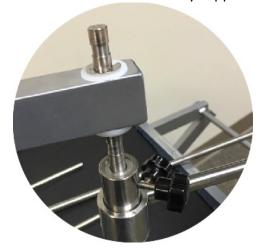
12. Place the LED light onto the support arm. Verify all the adjustment knobs are securely tightened. Failure to secure the adjustment knobs may result in damage to the equipment or injury to the operator/patient.
