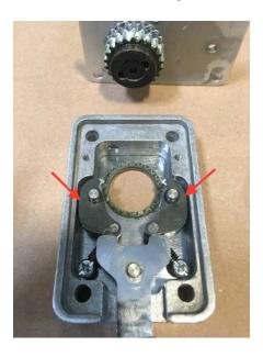
• Gently lift up on each tooth and remove the spring fastener.
