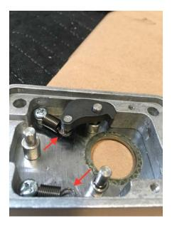
$\bullet\,$  Once both teeth are replaced, insert the locking lever . Rock the lever from left to right to secure it in place.
