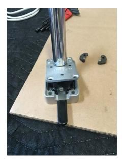
• Work the lever left and right to allow the gears to seat back into the assembly.
