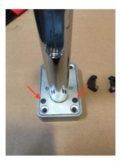
• Once the Allen screws are removed, use a flat head screw driver and gently pry the top portion of the ratchet assembly apart.
