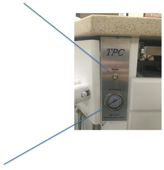
B. HANDPIECE PRESSURE GAUGE: Indicates pressure adjusted by the Drive-Air Control Knob. Avoid exceeding the manufacturer's recommended handpiece pressure. (30 - 35 PSI for most Highspeed Handpieces)
